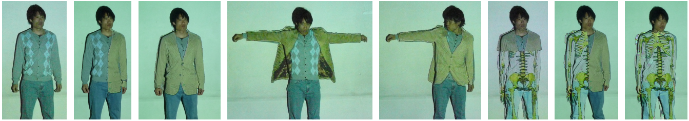
Figure 1: Dynamic dress-up simulator in the real-world. The color and patterns of user's clothes (leftmost image) are overwritten with projected images, and changed into a new looking. The new clothes are fitted with user's active motions. This effect can be seen with our own eyes, through no additional displays. Moreover, this system can achieve entertainment effects like a see-through human.
